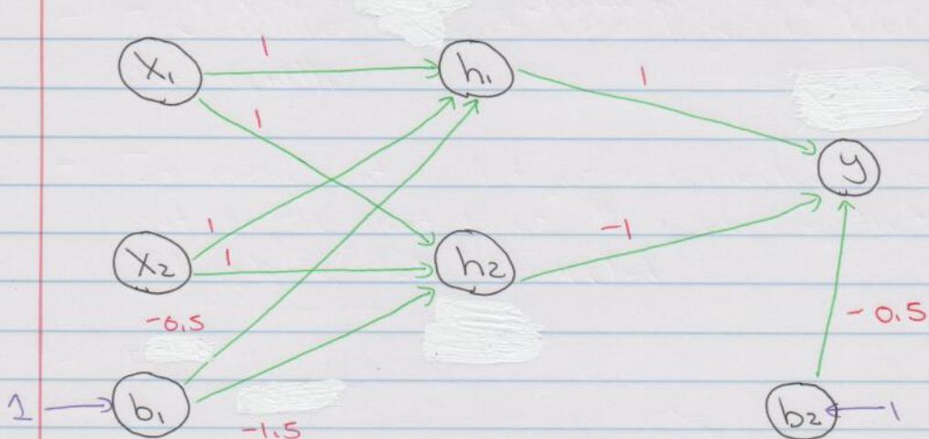
Here, we will introduce an **activation function**. An **activation function** is just a non-linear function applied to a node to get its output value from its inputs.
